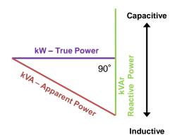
Power factor is the ratio of the demand for True Electric Power (kW) divided by the demand for Apparent Power (kVA).
